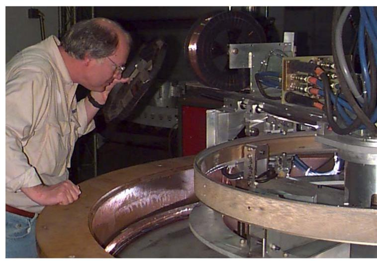
Fig. 1. Photograph of semiautomatic rotary remote welding system
