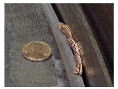
Fig. 2. Copper wire in joint
